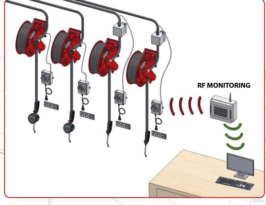
The data connection between dispensers devices and control unit takes place via RF Radio Frequency signal
