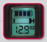
Grease level flashes when low grease condition occurs
