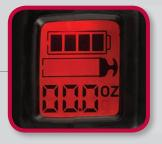
Display flashes red when the gun loses prime or runs out of grease
